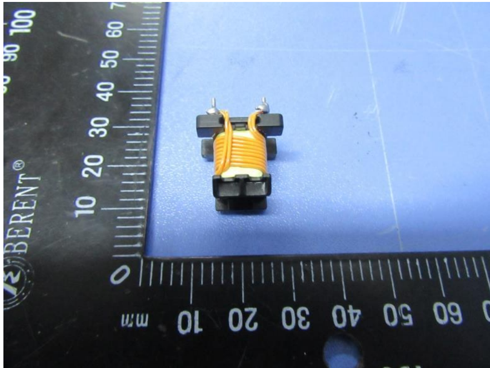
Figure 24. Transformer internal view top (N3 winding) for model 51500773
